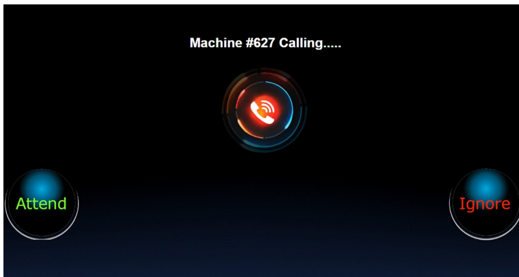
Figure 5. The screen demonstrates what the test participant saw when the machine called the operator to report factory critical condition.
